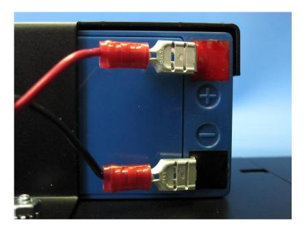
The red wire must match the red terminal (+) and the black wire the black terminal (-). *Failure to connect the battery properly could damage the Cv3*.
