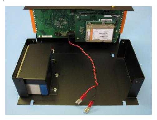
Remove the 4-40 locknuts and battery bracket:
