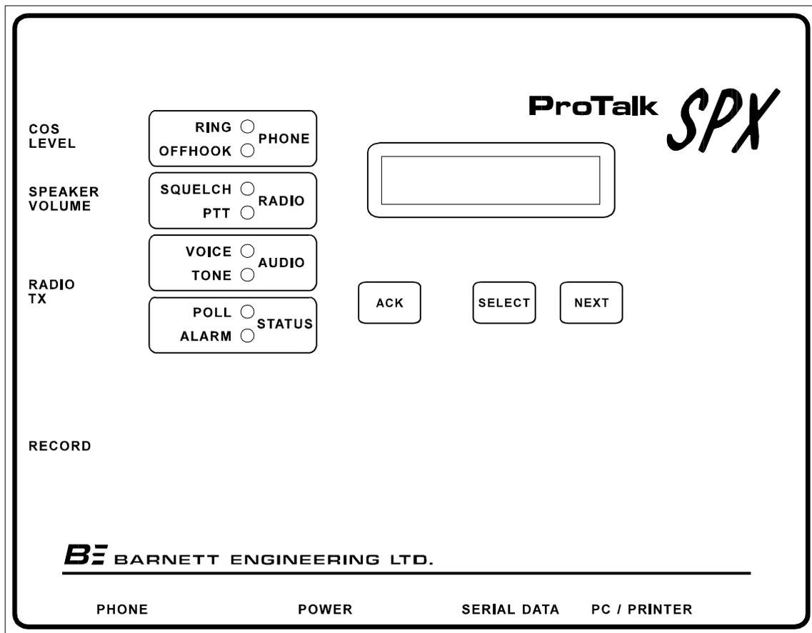
Figure 3 ProTalk SPX Front Panel
