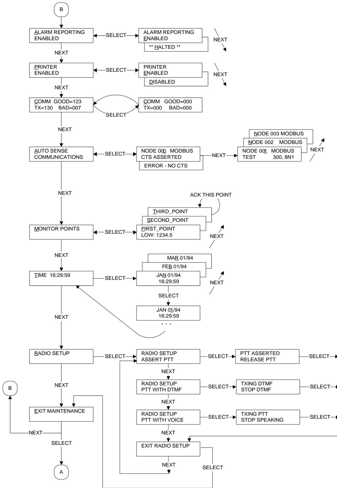
Figure 7b Maintenance Mode - Flowchart
