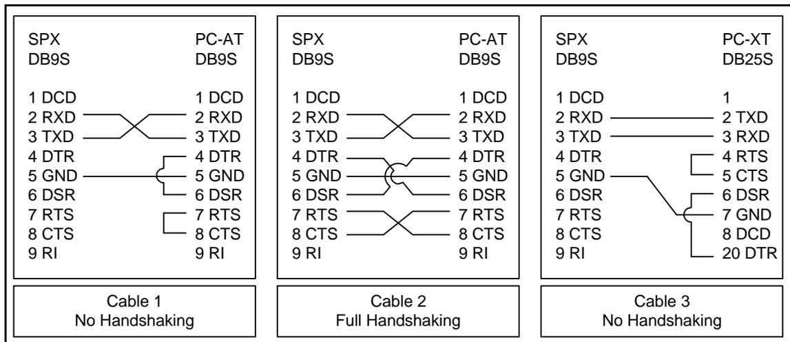
**Figure 4 PC Serial Connections**
