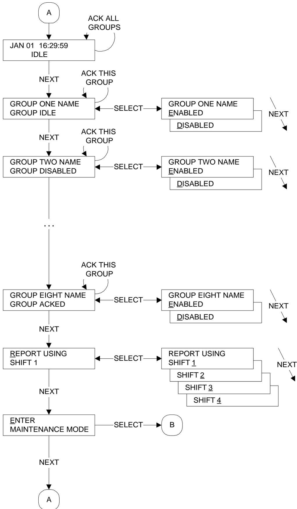
Figure 6a Front Panel Operation - Flowchart
