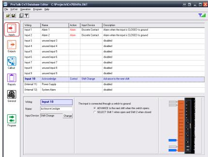
By default, the input (either the + or – terminals) should be grounded using a switch of some kind (toggle, push-button, relay, etc.). The shift will advance when the input detects that it is open. Any subsequent shift advances requires that the input be grounded and then opened again. To identify what shift is currently being used, the input 10 LED on the top of the Cv3 will be off for shift 1, solid green for shift 2, flashing green for shift 3 and flashing orange for shift 4.
