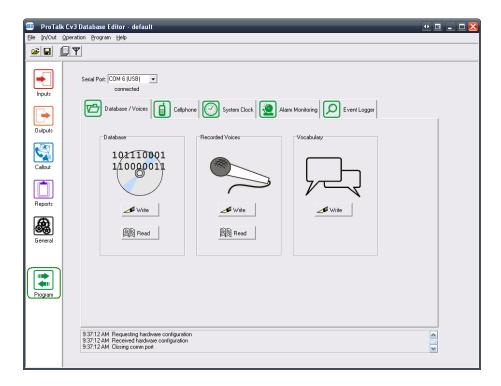
Select the 'Database/Voices' tab and press the 'Read' button under the 'Database' heading. The Cv3 configuration has now been loaded into the software. Press the 'Callout' button at the left-hand-side of the window:
