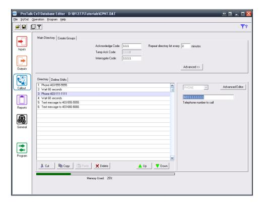
Once the number has been changed, press the 'Program' button and then the 'Write' button (under the 'Database' heading). The new number is now in the Cv3.
